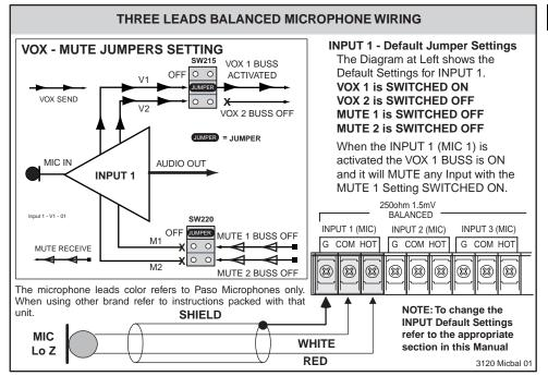
Fig. 10 - Balanced Microphone Input 1 Wiring
